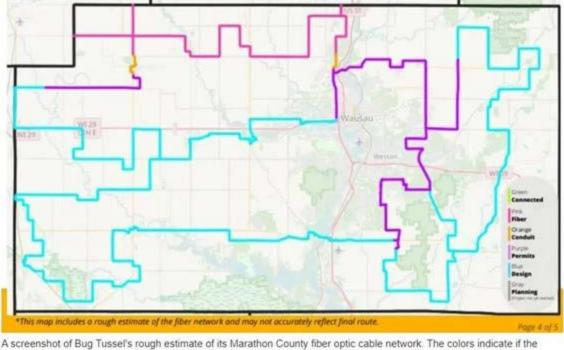
A screenshot of Bug Tussel's rough estimate of its Marathon County fiber optic cable network. The colors indicate if the section is at the stage where fiber is being laid (pink), where conduit cables are being laid (orange), where permitting is underway (purple) and design work is happening (blue). Courtesy Of Bug Tussel Wireless
